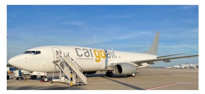
The AEI converted B737-800SF freighter offers a main deck payload of up to 52,700 lbs. (23,904 kg) and incorporates eleven full height 88" x 125" container positions, plus an additional position
